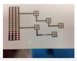
Simple Grid Structure printed on DMP
